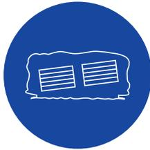
Store off the ground and with a minimum 50° slope (1:10) so that if rain penetrates the covering, water will drain away and not form a water pond.
