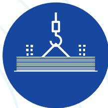
Use a spreader bar for long sheets. For small to medium size projects, without mechanical handling facilities, you can unload sheets by hand and pass them up to the roof one at a time.
