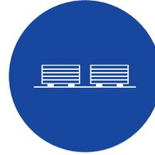
If material is not required for immediate use, stack them neatly and clear off the ground. Maintain a clear gap of 30 cm between sheet package and ground.
